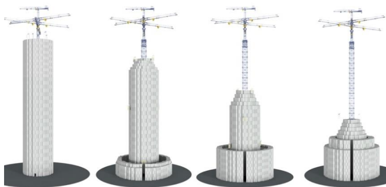
Figure 2.3.3 : Energy Vault Storage Method
